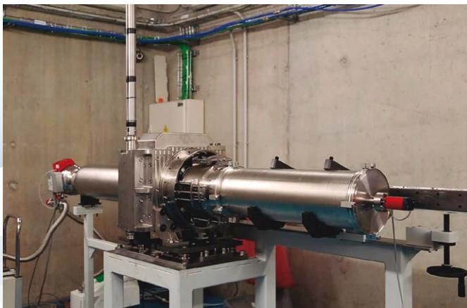
Remote Clamp (ESS) vacuum + remote handling
