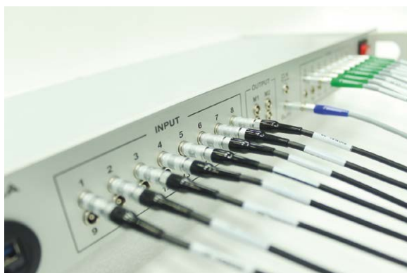
16 channels Digital Signal Processing System (FPGA)
