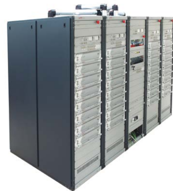
350kW liquid-cooled SSPA for CERN
