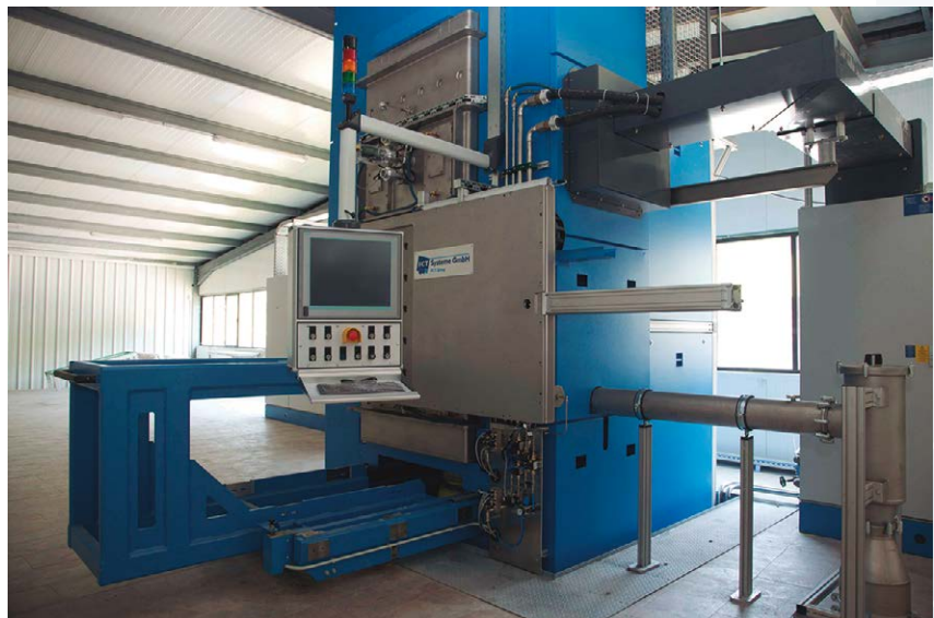
Large scale Spark Plasma Sintering (SPS)
