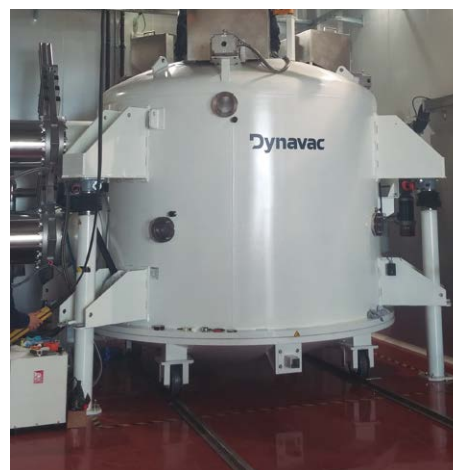
The OAJ vacuum chamber for aluminizing mirrors of up to 3m diameter
