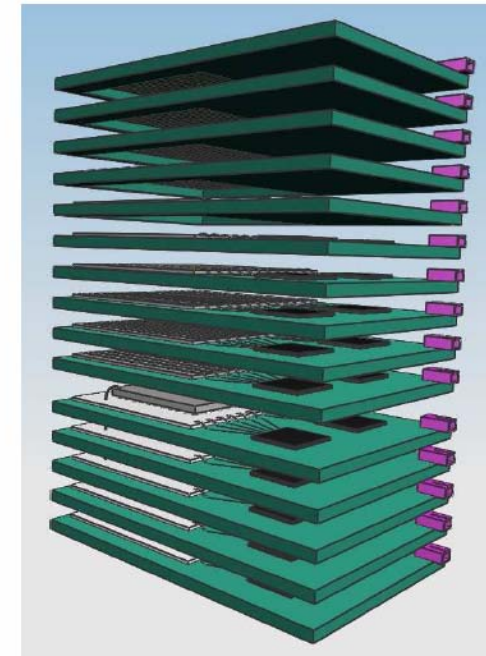
Figure 6. Schematic view of the global system, with the 15 sensing layers.
