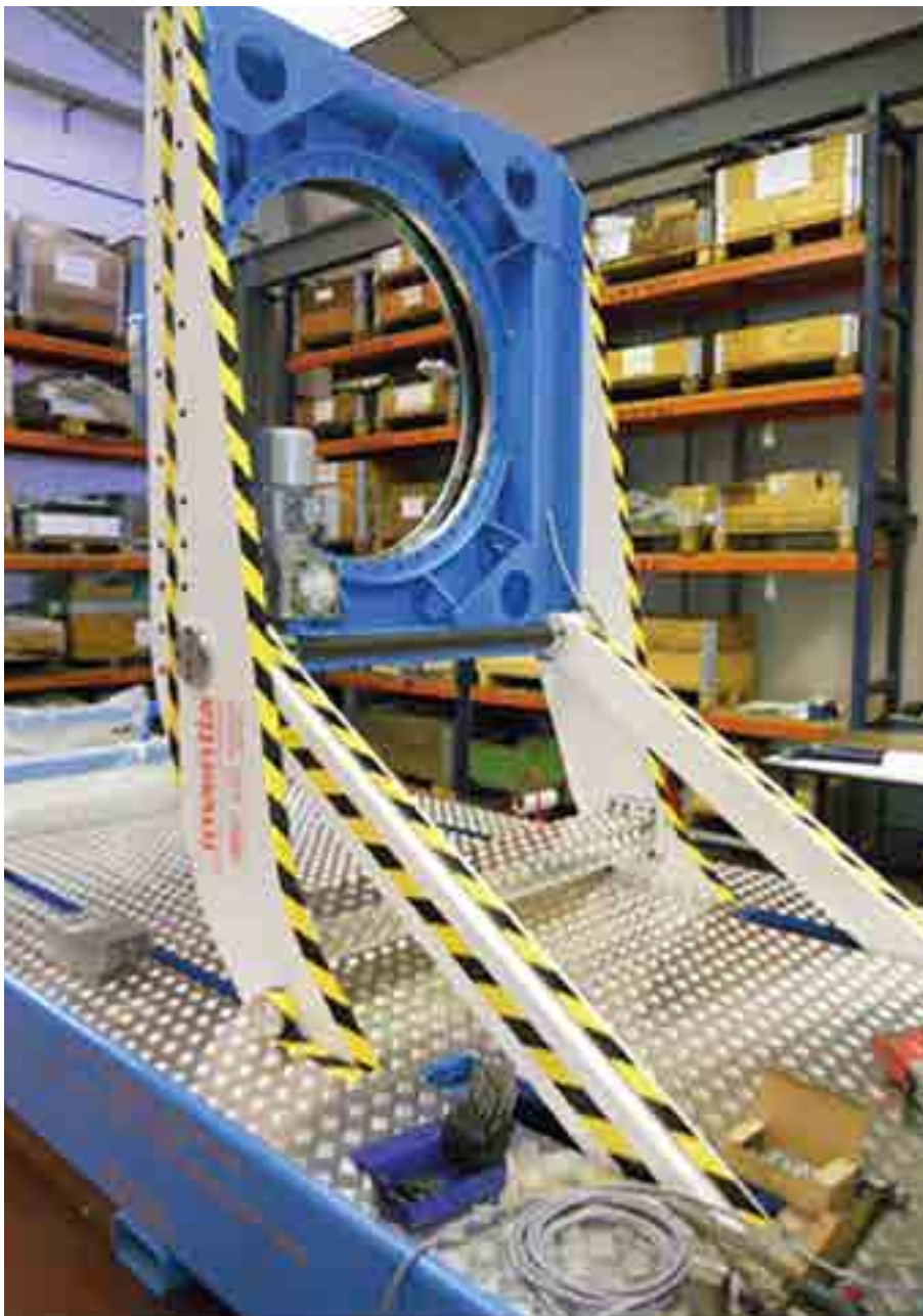
Automation and Robotics of Tooling. Special Machines. MGSE. SEOSAT Satellite Integration Tool
