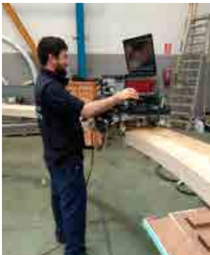
Qualification of UT inspection procedures for precompression rings (ITER)
