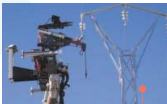
Technological exhibition on occasion of the NPC and HLG meetings of Málaga: Robot for live line maintenance in electrical networks.
